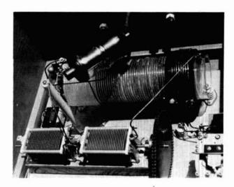
fig. 5. The interior view of the coupler housing illustrates the precautions taken with component placement as a result of high voltages present.
